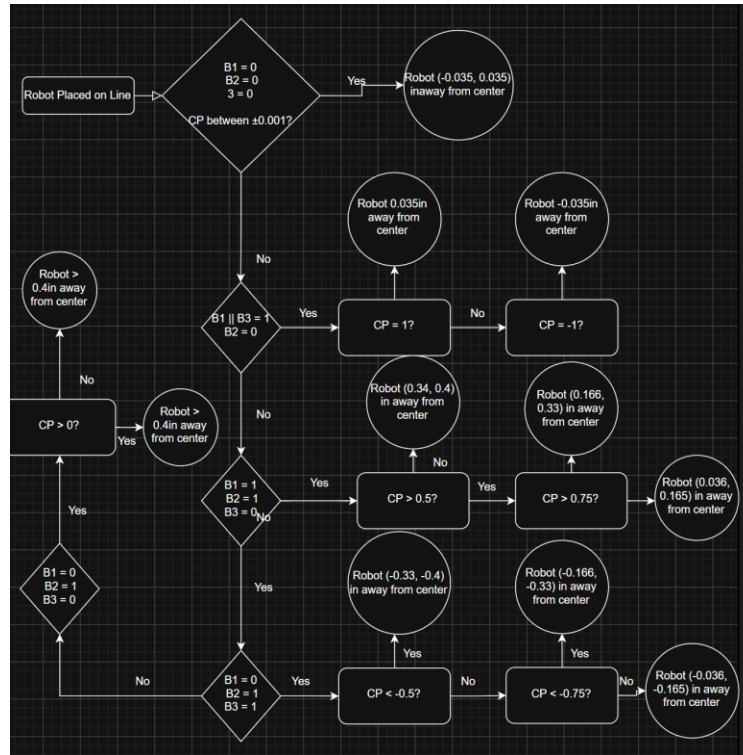
Fig 2.3.1 Binary Sensor Value to Robot Position From Center
